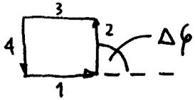
$$\Delta\varphi = \frac{2\pi}{4} \quad \therefore \quad \Delta C_o = \frac{\Delta\varphi \cdot \lambda}{2\pi} \Rightarrow \Delta C_o = \frac{2\pi \cdot \lambda}{4 \cdot 2\pi}$$
